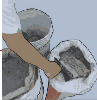
5. Mix CretePlus-Te + Cement + Sand (Optional)
