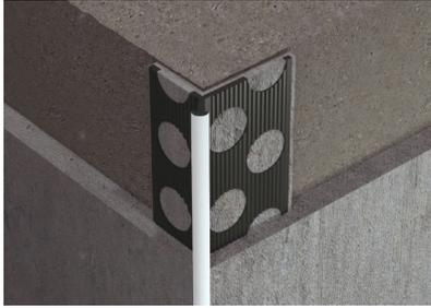
UPVC corner bead are installed at all type corners of clay brick/sand block wall and uneven shear wall which require thicker finishing.
